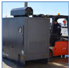
Anti-rollover forklift tunnels to ensure safe lifting and handling
